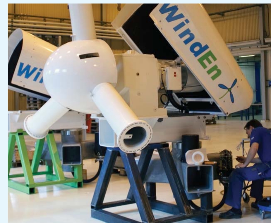
Above the platform, that makes maintenance easy and safe can be seen. To the right the production of WindEn45 at UFAB in Uddevalla, Sweden.
