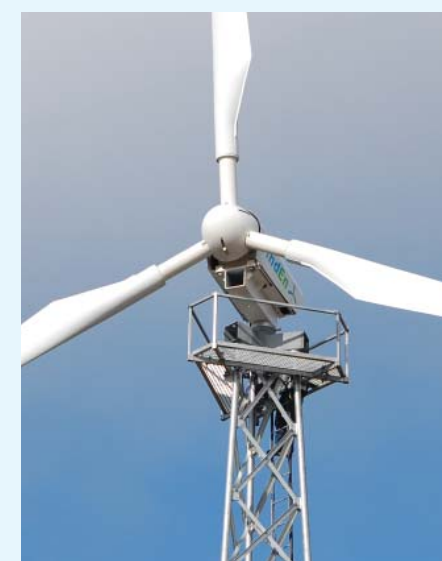
Above the platform, that makes maintenance easy and safe can be seen. To the right the production of WindEn45 at UFAB in Uddevalla, Sweden.
